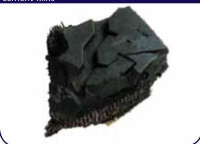
Figure 3: a CM tyre shredder produces a 50mm clean-cut tyre chip, ideal TDF for cement kilns
