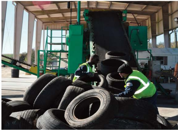
CM Dual Speed Shredder being loaded with truck tires.
